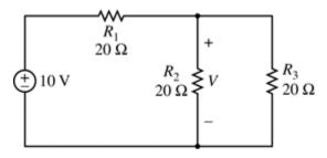
34. The closed electrical circuit shown consists of a generator and three resistors,  $R_1$ ,  $R_2$  and  $R_3$ . The electromotive force of the generator is 10 volts. Which of the following is the second resistor's voltage, V?
